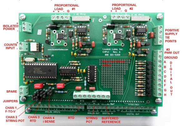
with the maximum voltage input. If maximum current is not a limitation, the factory settings should be adequate. That setting provides approximately 50% duty cycle at 2.5 volts in.
