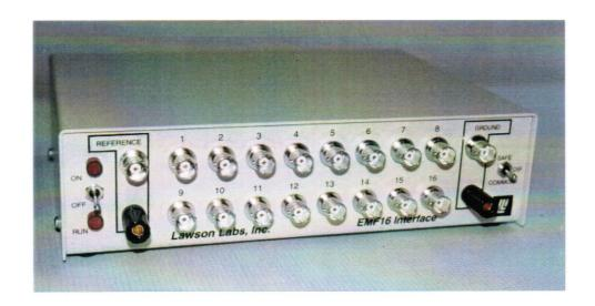
The EMF16 is a high-resolution, high input impedance, data acquisition system for electrochemistry applications. It connects to a PC serial port for presentation and storage of EMF data. The bundled software is written by electrochemists for electrochemistry. It allows up to 16 channels of data to be scanned and displayed and saved to the disk in real time.
